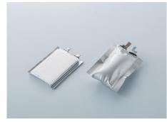
Left: A new battery Right: A battery after repeated charging and discharging
